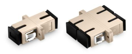
BLACKSTONE fiber adapters are constructed of engineered thermoplastic with precision zirconia ceramic split sleeves providing low loss fiber connections over high and low temperature extremes. SC adapters are suitable for any data center, central office, MDU, CATV, or PON cabling installations using SC connectors. SC adapters are available with mounting flanges or flangeless for higher density applications.
