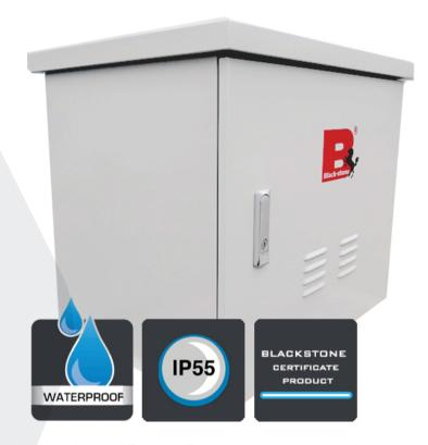
IP55 wall mount rack cabinet with a 450mm Depth. Outdoor wall data cabinet to house telecoms CATV or CCTV equipment. Cabinets include 19" profile with optional fans, heater, and floor mount plinth. Perfect wall or roof mount external data cabinet, providing IP55 protection against dust and water ingress. For Wall Mounting please use PN: BSC-OC"X (u size)"-6450-SS
